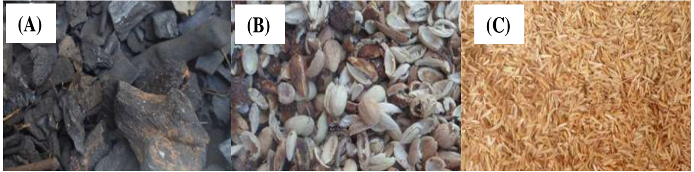
Figure 2. Biomass used for the gasification tests; (A) Charcoal, (B) Balanites aegyptiaca hulls, (C) rice husk.
